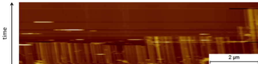
Figure B.8: Kymograph representing the topographic changes of a single scan line over time during the tip-induced formation of a scratch in the nanoparticle layer.
