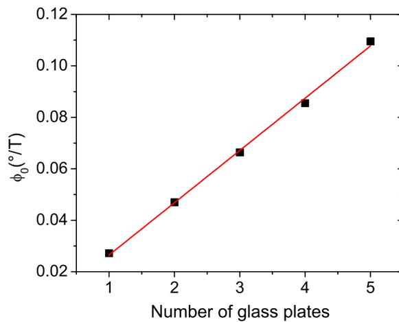
**Figure 3.** Faraday rotation in  $\text{deg T}^{-1}$  versus the borosilicate glass thickness, expressed in number of glass plates.
