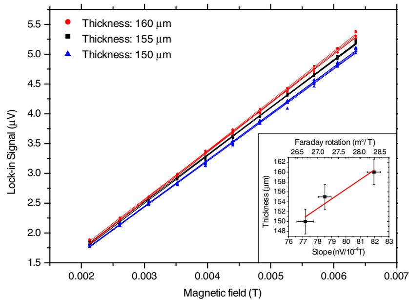
**Figure 2.** Lock-in signal versus applied magnetic field for three samples with different thicknesses during the measurement of Faraday rotation in borosilicate glass. In the inset, the average slopes per sample versus the sample thickness and the corresponding Faraday rotation in  $\text{mdeg T}^{-1}$ .
