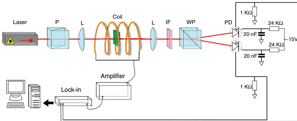
**Figure 1.** Experimental setup. After passing the polarizer P, the laser beam is focused on the sample by a lens L. It is then made parallel again with a second lens and then traverses an interference bandpass filter IF. Finally, it is directed through the Wollaston prism WP at the photodiodes (PD). The lock-in drives the magnetic coil through the amplifier and detects the signal from the PD at the same frequency.
