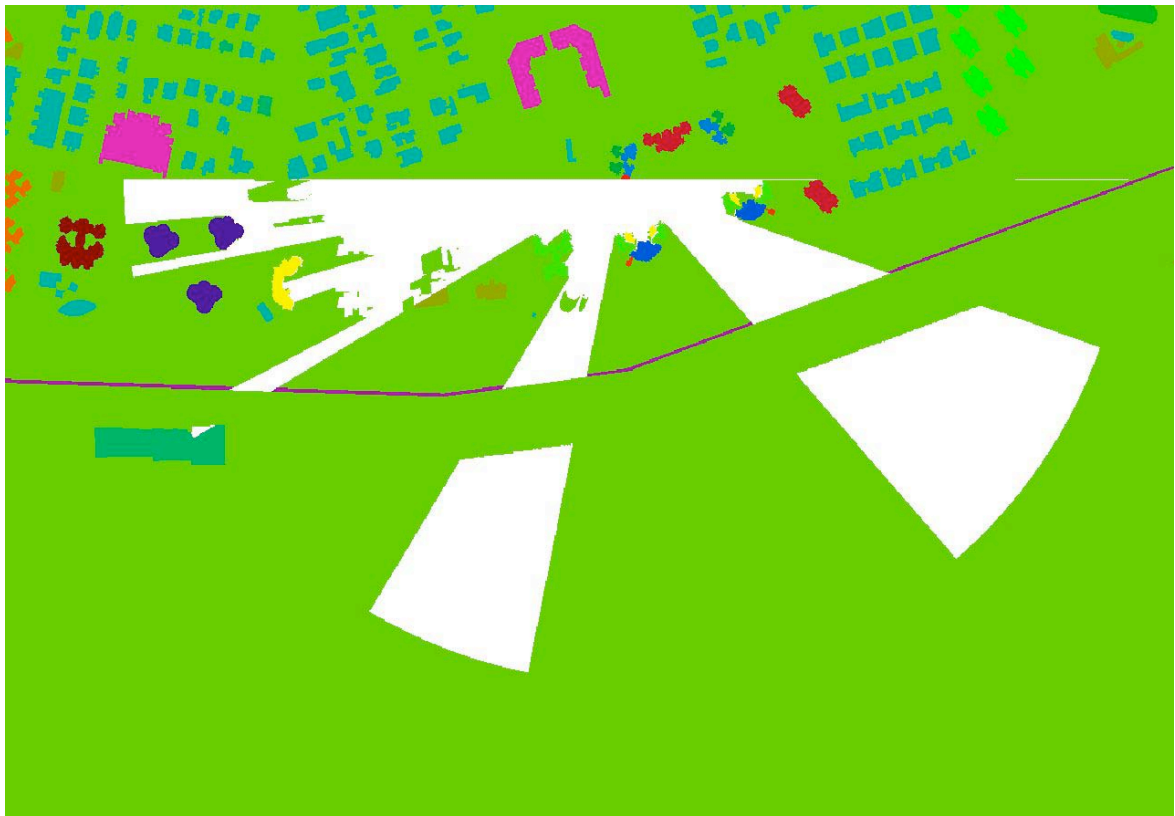
Figure 15: The viewshed from the particular observation point is displayed in white. Note the effect of the obstructing neighbouring buildings.
