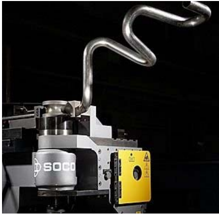
Fig. 130 NC Controlled Pipe Bending.
