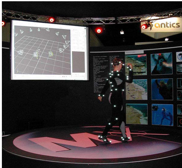
Fig. 42 A dancer wearing a suit used in optical Motion Capture Systems.
