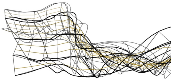
Fig. 133 The basic steel structure (black) with the secondary steel elements (gray) and the ropes (yellow).
