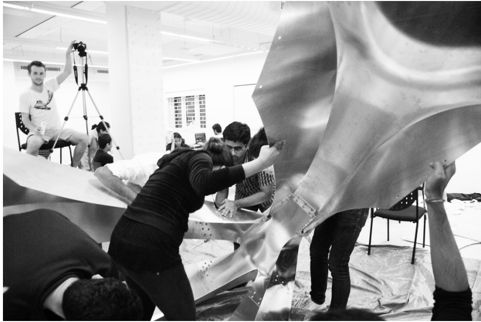
Figure 81. 2m long aluminium polyhedron, folded and assembled in 6 hours by a group of 15 students. Image courtesy (Chandra et al. 2014)
