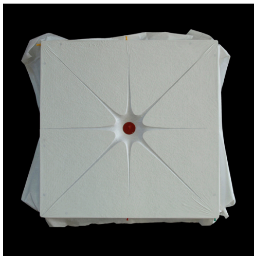
Figure 1.6: Fabric is pre-stressed and vacuum applied (West, 2011)
