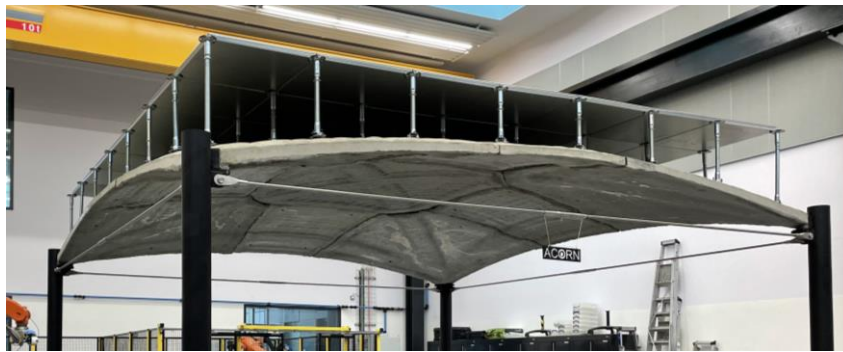
Figure 1: ACORN's full-scale segmented concrete thin-shell prototype © Paul Shepherd
