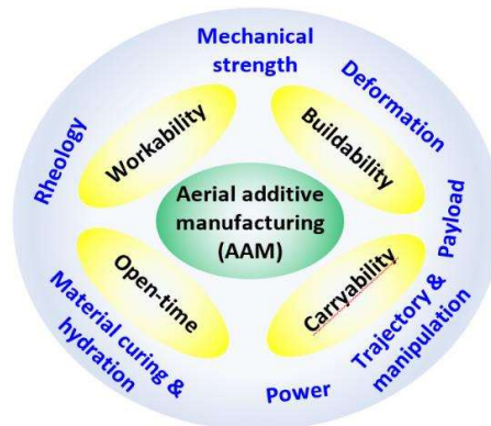
Fig. 3. Four main factors - ‘carryability’, ‘workability’, ‘buildability’ and ‘open-time’ proposed by the authors that must be optimized to enable AAM.
