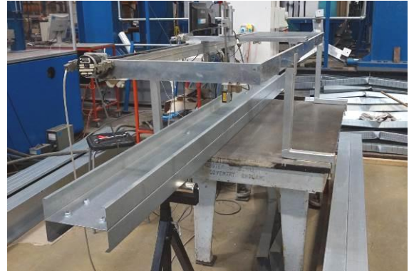
Fig.6 Imperfection measurement set-up
