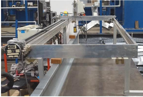
Fig.6 Imperfection measurement set-up
