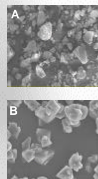
Fig. 2. SEM micrographs of (A) micronised and (B) SAXS budesonide particles
