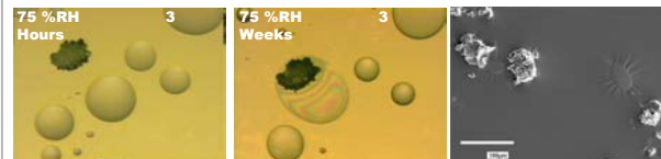
Figure 3: Incomplete re-crystallisation of isolated amorphous lactose particles upon exposures to a relatively high 75%RH.
