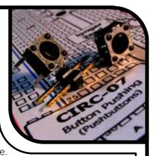
This is included because an Arduino doesn't sense the same way we do (ie button pressed, button unpressed). Instead it looks at the voltage on the pin and decides whether it is HIGH or LOW. The button is set up to pull the Arduino's pin LOW when it is pressed, however, when the button is unpressed the voltage of the pin will float (causing occasional errors). To get the Arduino to reliably read the pin as HIGH when the button is unpressed, we add the pull up resistor.
