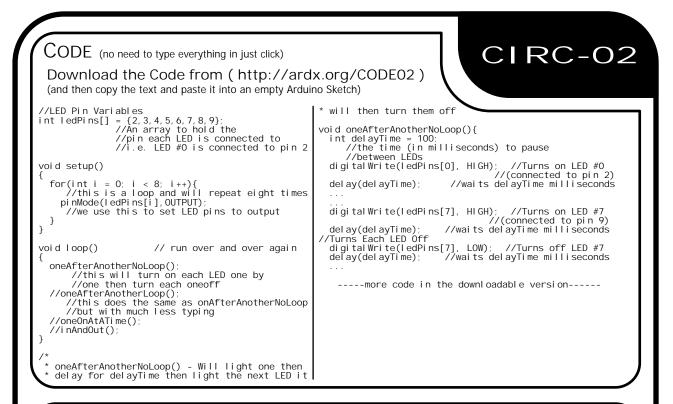
Some LEDs Fail to Light It is easy to insert an LED backwards. Check the LEDs that aren't working and ensure they the right way around. Operating out of sequence With eight wires it's easy to cross a couple. Double check that the first LED is plugged into pin 2 and each pin there after. Starting Afresh Its easy to accidentally misplace a wire without noticing. Pulling everything out and starting with a fresh slate is often easier than trying to track down the problem.
