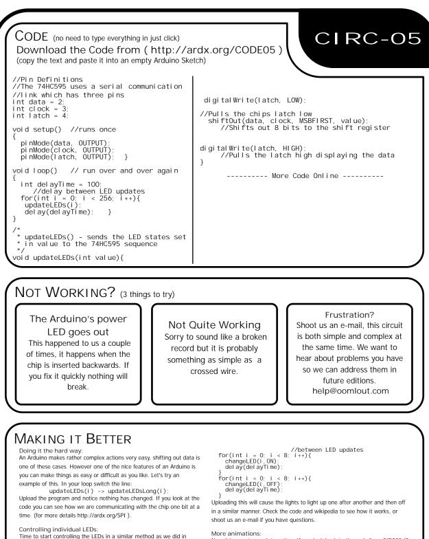
Time to start controlling the LEDs in a similar method as we did in CIRC02. As the eight LED states are stored in one byte (an 8 bit value) for details on how this works try http://ardx.org/BINA. An Arduino is very good at manipulating bits and there are an entire set of operators that help us out. Details on bitwise maths ( http://ardx.org/BITW ).
