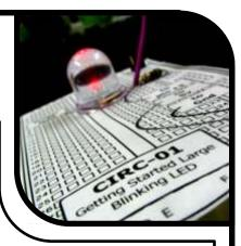
everything in. Once the circuit is assembled you'll need to upload the program. To do this plug the Arduino board into your USB port. Then select the proper port in Tools > Serial Port > (the comm port of your Arduino). Next upload the program by going to File > Upload to I/O Board (ctrl+U). Finally, bask in the glory and possibility that controlling lights offers.
