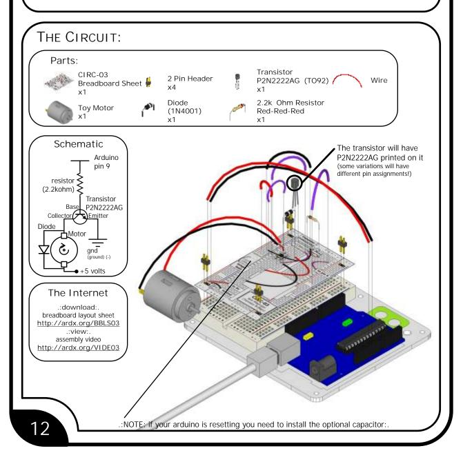
CIRC-03  $\mathsf{CODE}$  (no need to type everything in just click) Download the Code from (http://ardx.org/CODE03) (then simply copy the text and paste it into an empty Arduino Sketch) int motorPin = 9; //pin the motor is connected to void setup() //runs once pinMode(motorPin, OUTPUT); int onTime = 2500; int offSpeed = 50; // a number between //0 (stopped) and 255 (full speed) int offTime = 1000; void loop() // run over and over again motorOnThenOff();
