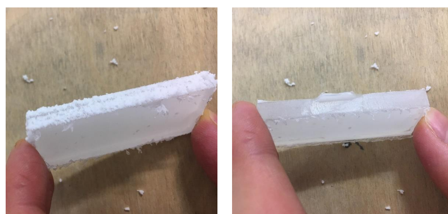
Figure 5. (a) The first test cut made on the CNC machine. (b) A better finish on subsequent test cuts after specific changes are implemented.
