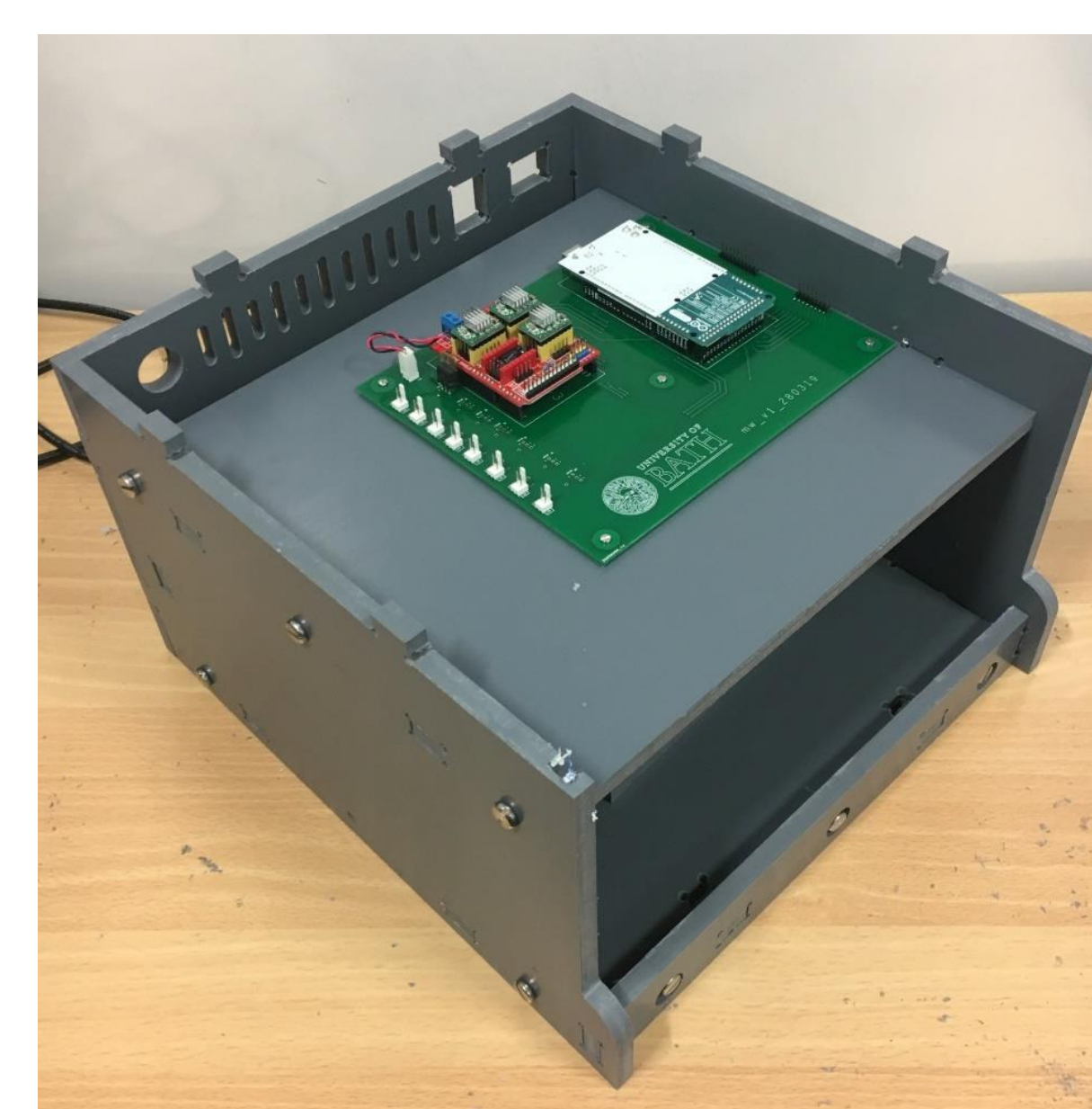
Figure 7. The PCB with the CNC Shield and Arduino is mounted inside of the enclosure.
