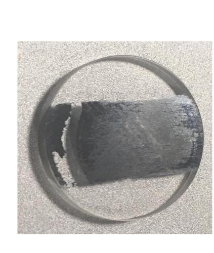
30 nm of aluminium (AI) was deposited onto 15 diameter quartz mm windows using the thermal evaporation method.
