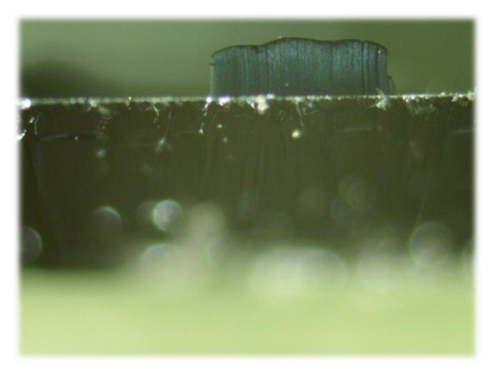
Growth heights of every sample were measured using a microscope and compared to the conditions of time, temperature and pressure varied in the CVD chamber.
