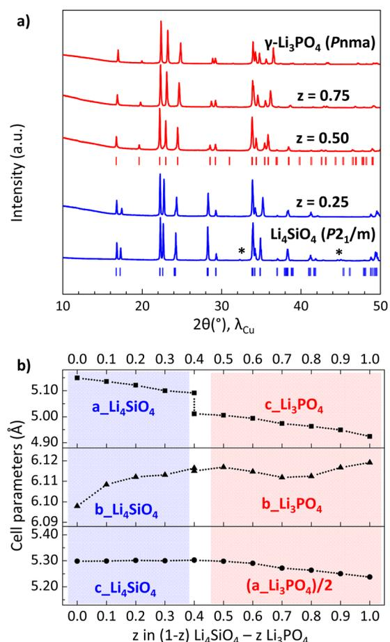
**Figure 2.** (a) XRPD patterns of powders obtained for the Li<sub>4</sub>SiO<sub>4</sub>–Li<sub>3</sub>PO<sub>4</sub> system. Li<sub>4</sub>SiO<sub>4</sub>-based patterns are in blue; Li<sub>3</sub>PO<sub>4</sub>-based patterns are in red. Asterisks (\*) indicate superstructure peaks. (b) Variation of lattice parameters as a function of *z* in (1–*z*)Li<sub>4</sub>SiO<sub>4</sub>–(*z*)Li<sub>3</sub>PO<sub>4</sub>.
