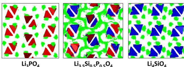
**Figure 12.** MD density plots of mobile lithium ions (green) overlaid on the tetrahedral framework structure ( $\text{PO}_4$ , red;  $\text{SiO}_4$ , blue) of  $\text{Li}_3\text{PO}_4$ ,  $\text{Li}_{3.5}\text{Si}_{0.5}\text{P}_{0.5}\text{O}_4$ , and  $\text{Li}_4\text{SiO}_4$ .
