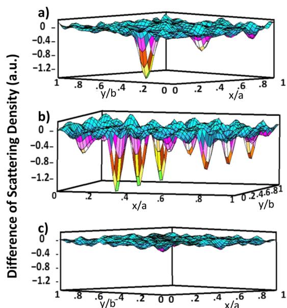
Figure 4. Fourier-transformed scattering density difference maps (at  $z = 0.7$ ) from refinements of  $\text{Li}_{3.5}\text{Si}_{0.5}\text{P}_{0.5}\text{O}_4$  neutron diffraction data (a) in the absence of Li1, (b) in the absence of Li2, and (c) with both Li1 and Li2.
