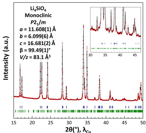
Figure 3. Full pattern profile matching of XRPD pattern of  $\text{Li}_4\text{SiO}_4$ : red dots, experimental data; black line, profile matching; blue bar, Bragg positions of the small cell; green bar, Bragg positions of the 7-fold super cell.
