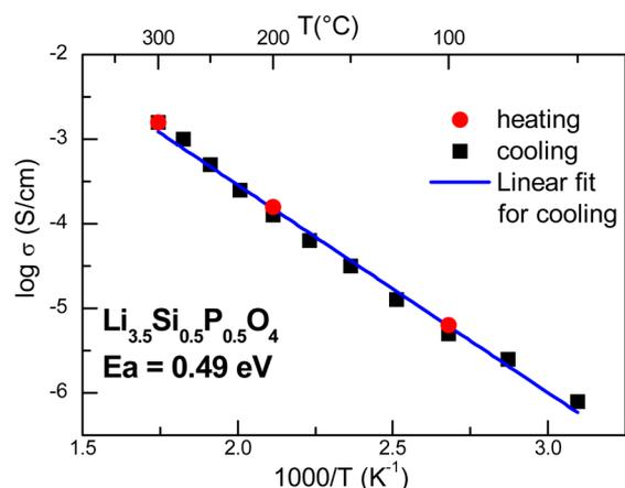
**Figure 10.** Arrhenius plot from AC impedance measurements for  $\text{Li}_{3.5}\text{Si}_{0.5}\text{P}_{0.5}\text{O}_4$  (as a representative example). Data were recorded upon heating (red circles) and cooling (black squares). The activation energy was derived from a linear fit of data from cooling process (blue line).
