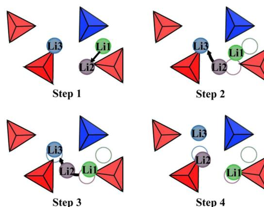
**Figure 14.** MD simulation snapshots of  $\text{Li}$ -ion positions in  $\text{Li}_{3.5}\text{Si}_{0.5}\text{P}_{0.5}\text{O}_4$  showing the cooperative knock-on like mechanism: the migrating interstitial  $\text{Li}^+$  (green) displaces another  $\text{Li}^+$  (purple) toward a neighbor site which in turn leads to further  $\text{Li}^+$  (blue) migration ( $\text{PO}_4$ , red;  $\text{SiO}_4$ , blue).
