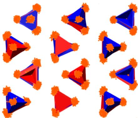
**Figure 13.** Density plots of oxygen atoms (orange) during the MD simulation overlaid on the tetrahedral framework structure of  $\text{Li}_{3.5}\text{Si}_{0.5}\text{P}_{0.5}\text{O}_4$  ( $\text{PO}_4$ , red;  $\text{SiO}_4$ , blue).
