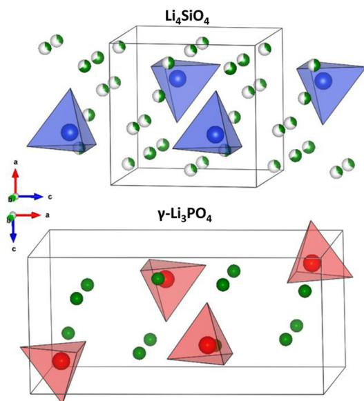
**Figure 1.** Schematic representations of the crystal structures of the end member phases  $\text{Li}_4\text{SiO}_4$  (subcell) and  $\gamma\text{-Li}_3\text{PO}_4$ . Key:  $\text{SiO}_4$  and  $\text{PO}_4$ , blue and red tetrahedra; lithium, green. Partially occupied Li sites are represented by partial shading. Unit cells are shown as solid lines.
