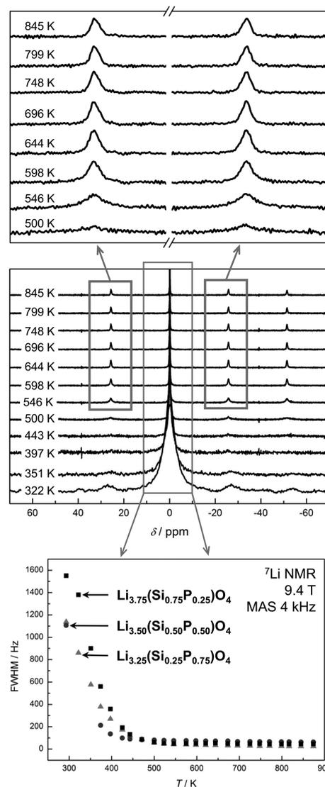
**Figure 6.**  $^7\text{Li}$  VT MAS (4 kHz) NMR signals at 9.4 T. The middle graph shows the full spectra for  $\text{Li}_{3.25}\text{Si}_{0.25}\text{P}_{0.75}\text{O}_4$  with a zoom of the first rotational sidebands at high temperatures (top). Temperature-dependent  $^7\text{Li}$  fwhm values of the CT signals are depicted at the bottom for all samples.
