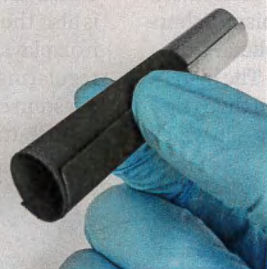
A flexible electroplated lithium cobalt oxide battery electrode can be rolled up.
