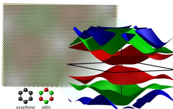
**Figure 1** Moiré pattern of graphene on hexagonal boron nitride (hBN) and the electronic miniband structure of bilayer graphene on hBN [4].
