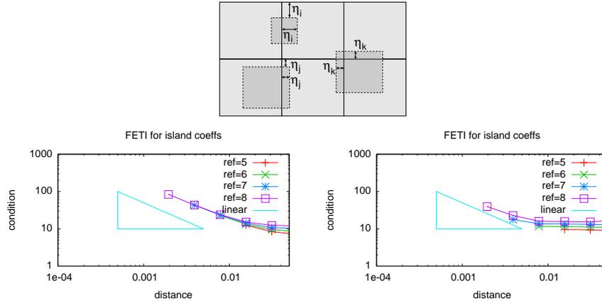
**Fig. 3** Upper: Sketch of coefficient “islands” cutting through edges and crosspoints of the subdomain partitioning. Lower left: Condition numbers for “edge islands”. Lower right: Condition numbers for “crosspoint islands”.
