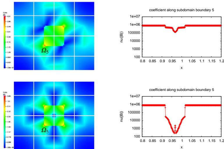
**Fig. 4** Upper: Case 1. Lower: Case 2. Left:  $|\mathbf{B}|$ -field, subdomain partition. Right: Coefficient  $\nu(|\mathbf{B}|)$  plotted along the boundary of subdomain  $\Omega_5$ .
