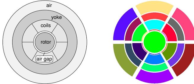
**Fig. 1** Left: Model of an electric motor. Right: Possible subdomain partitioning (explosive view).
