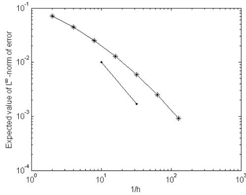
Figure 3-4:  $\mathbb{E}[\|u_{h^*} - u_h\|_{L^\infty(D)}]$  versus  $1/h$  for model problem (3.18) with  $d = 2$  and 2-norm exponential covariance with  $\mu = 0, \lambda = 0.3, \sigma^2 = 1$  and  $h^* = 1/256$ . The gradient of the (non-marked) solid line is  $-3/2$ .
