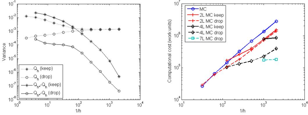
Figure 4-7: Left: Plot of  $\mathbb{V}[M^{(1)}(u_h)]$  and  $\mathbb{V}[M^{(1)}(u_h) - M^{(1)}(u_{2h})]$ , for (3.18) with  $d = 1$ ,  $\lambda = 0.01$ ,  $\sigma^2 = 1$ ,  $R_\ell = h_\ell^{-1}$ ,  $h^* = 1/4096$ ,  $R^* = 4096$  and  $x^* = 2049/4096$ . Right: Plot of cost versus  $1/h$  for a fixed tolerance of the sampling error of  $\delta = 10^{-3}$ , for the same model problem.
