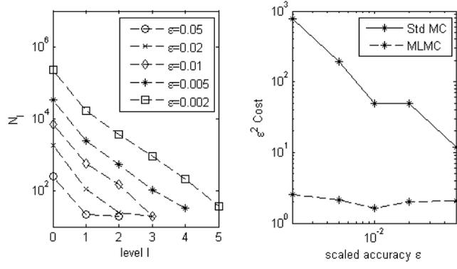
Figure 4-5: Left: Number of samples  $N_\ell$  per level. Right: Plot of the cost scaled by  $\epsilon^{-2}$  of the MLMC and standard MC estimators for  $d = 2$ , with  $\lambda = 0.3$  and  $\sigma^2 = 1$ . The coarsest mesh size in all tests is  $h_0 = 1/8$ .
