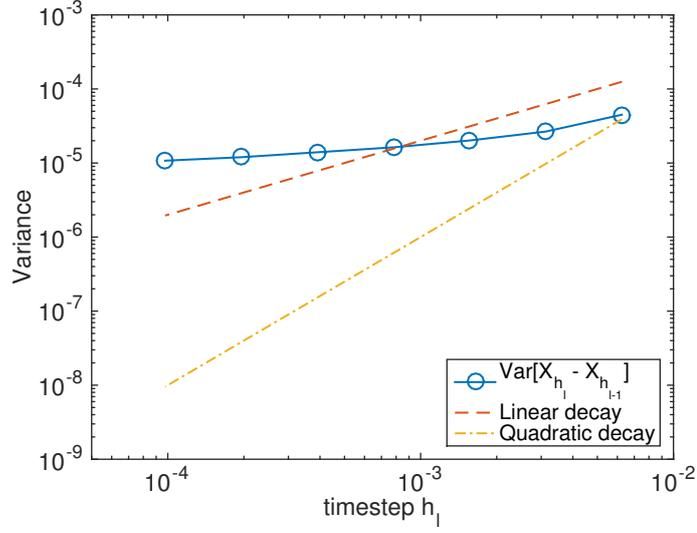
Figure 5-3: Symplectic Euler - Boundary Conditions and no special treatment
