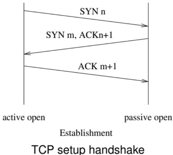
The initial SYN can be lost just like any other segment, so we need to ACK it independently of the first data byte, which comes later;
