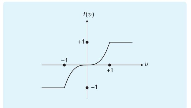
**FIGURE 11** Saturating nonlinearity  $f$ . The feedback  $u = -f(x)$  applied to the integrator  $\dot{x} = u$  yields asymptotic stability in the large but not global exponential stability.
