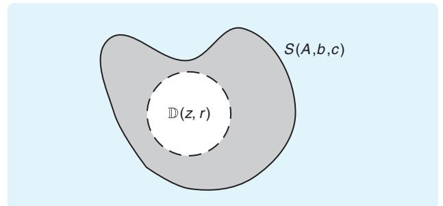
**FIGURE 10** A disc  $\mathbb{D}(z, r)$  of stabilizing complex gains. If  $(A, b, c)$  is stabilizable and detectable, then, by Lemma 6, the disc  $\mathbb{D}(z, r)$  is contained in the set  $S(A, b, c)$  of stabilizing complex gains if and only if the rational function  $1 + 2rc^*(sI - (A - \kappa bc^*))^{-1}b$  is positive real, where  $\kappa := z - r$ .
