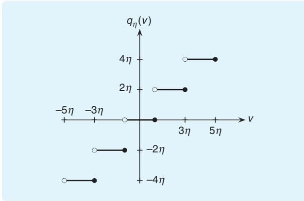
**FIGURE 8** Uniform quantizer  $q_\eta$ . For every  $v \in \mathbb{R}$  there exists a unique integer  $m \in \mathbb{Z}$  such that  $v \in ((2m-1)\eta, (2m+1)\eta]$  and the quantizer  $q_\eta$  maps  $v$  to  $2m\eta$ .
