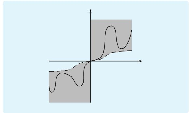
**FIGURE 16** **(H2)**-type sector. Inequality (38) holds if and only if the graph of the nonlinearity  $\Phi$ , illustrated here in the case of a singleton-valued map for simplicity, lies in the shaded region bounded by the vertical axis and the curve given by the graph of  $\varphi$  and its reflection through the origin.
