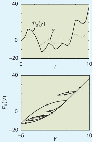
**FIGURE S5** Example of Prandtl hysteresis. Consider the Prandtl operator  $\mathcal{P}_\xi$  defined in (S12) with  $\xi = 0$  and measure  $\mu$  given by  $\mu(E) = \int_E \chi_{[0,5]}(\sigma) d\sigma$ , where  $\chi_{[0,5]}$  is the indicator function of the interval  $[0,5]$ . The plots depict the response  $\mathcal{P}_0(y)$  to a continuous, piecewise linear input  $y$ .
