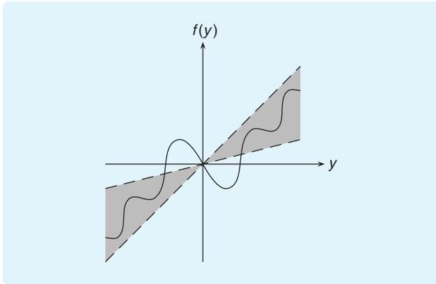
**FIGURE 4** Nonlinearity  $f$  satisfying a generalized sector condition. The points  $(y, f(y))$  of the graph of  $f$  are contained in the shaded area, for all  $|y|$  sufficiently large.
