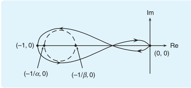
**FIGURE 12** Nyquist diagram of  $\mathbf{G}(s) = 10/(s^3 + 5s^2 + 4s - 10)$  and the disc  $D(\alpha, \beta)$  with  $\alpha = 1.07$  and  $\beta = 1.5$ . The Nyquist diagram of  $\mathbf{G}$  does not intersect the disc  $D(\alpha, \beta)$  and encircles it once in the counterclockwise sense. Therefore, by statement i) of Lemma 10,  $(1 + \beta\mathbf{G})(1 + \alpha\mathbf{G})^{-1}$  is positive real.
