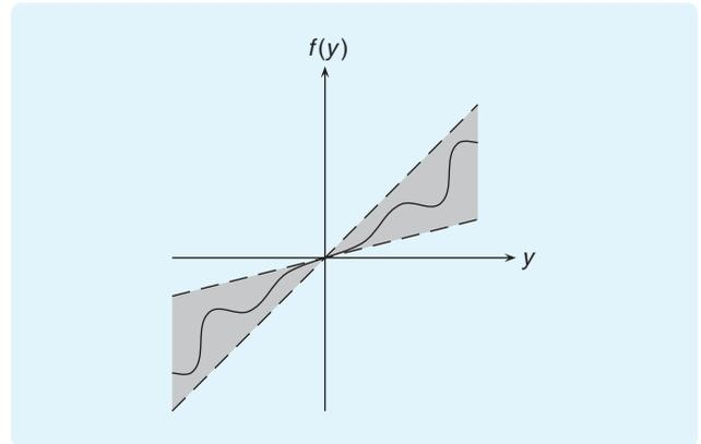
**FIGURE 2** Sector-bounded nonlinearity  $f$ . The graph of  $f$  is contained in the shaded sector determined by two lines through the origin.
