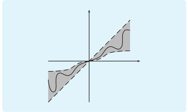
**FIGURE 15** **(H1)**-type sector. Inequalities (37) hold if and only if the graph of the nonlinearity  $\Phi$ , illustrated here in the case of a singleton-valued map for simplicity, lies in the shaded region bounded by the line of slope  $\beta - \delta$  through the origin and the curve given by the graph of  $\varphi$  and its reflection through the origin.
