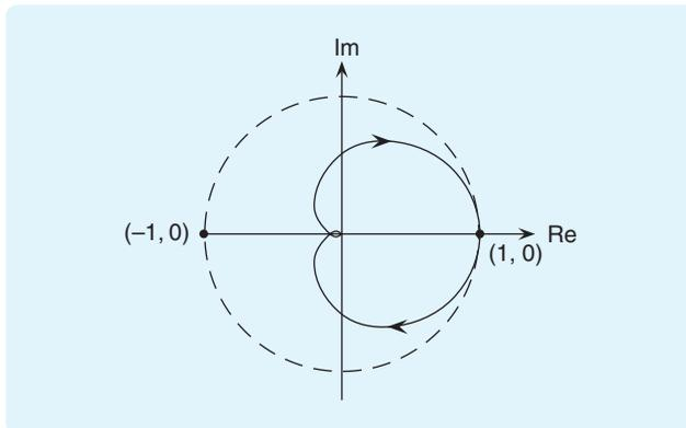
**FIGURE 13** The Nyquist diagram of  $\mathbf{G}(s) = 10/(s^3 + 7s^2 + 16s + 10)$  and the closed unit disc  $\bar{D}(-1, 1)$ . The Nyquist diagram of  $\mathbf{G}$  is contained in the closed disc  $\bar{D}(-1, 1)$ , and thus, by statement ii) of Lemma 10,  $(1 + \mathbf{G})(1 - \mathbf{G})^{-1}$  is positive real.
