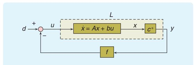
**FIGURE 3** Lur'e system. This system consists of a linear system  $L$  and a static nonlinearity  $f$  with exogenous input  $d$ , representing either a reference or disturbance signal.
