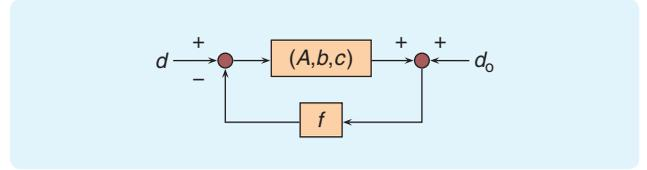
**FIGURE 20** Lur'e system. The linear system  $(A, b, c)$  is in the forward path, the nonlinearity  $f$  is in the negative feedback path, the exogenous input is  $d$ , and the output disturbance is  $d_0$ .
