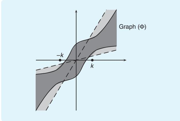
**FIGURE 14** Set-valued  $\Phi$  satisfying the sector condition (34) with  $K = [-k, k]$ . For every  $v \in \mathbb{R}$  such that  $|v| > k$  and every  $w \in \Phi(v)$ , the point  $(v, w)$  lies in the sector given by the shaded area bounded by the two dashed lines passing through the origin.
