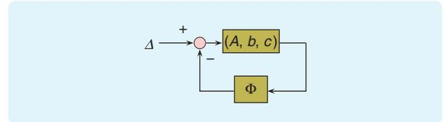
**FIGURE 6** A system of Lur'e type in a set-valued setting. The linear system  $(A, b, c)$  is interconnected with the set-valued nonlinearity  $\Phi$ , and the resulting feedback system is subjected to a set-valued exogenous input  $\Delta$ .
