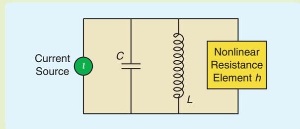
**FIGURE S1** Example from circuit theory. A parallel connection of a current source, capacitor, inductor, and nonlinear resistive element  $h$ .
