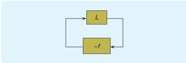
**FIGURE 1** A classical Lur'e system. The negative feedback interconnection consists of a linear system  $L$  in the forward path and a static, sector-bounded nonlinearity  $f$  in the feedback path.
