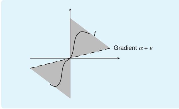
**FIGURE 18** PID control application. Sector-bounded static nonlinearity. The graph of  $f$  is required to lie in the shaded region bounded by the vertical axis and the line of slope  $\alpha + \varepsilon$  through the origin.
