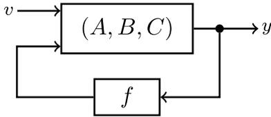
Fig. 1.1. Lur'e system with linear part  $(A, B, C)$ , nonlinearity  $f$ , output  $y$  and input  $v$ .
