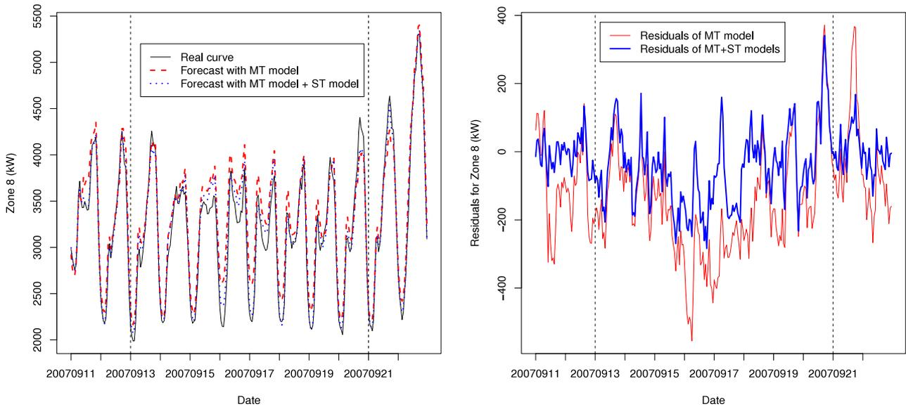
Fig. 2. Short term correction effects for zone 8 over a week.
