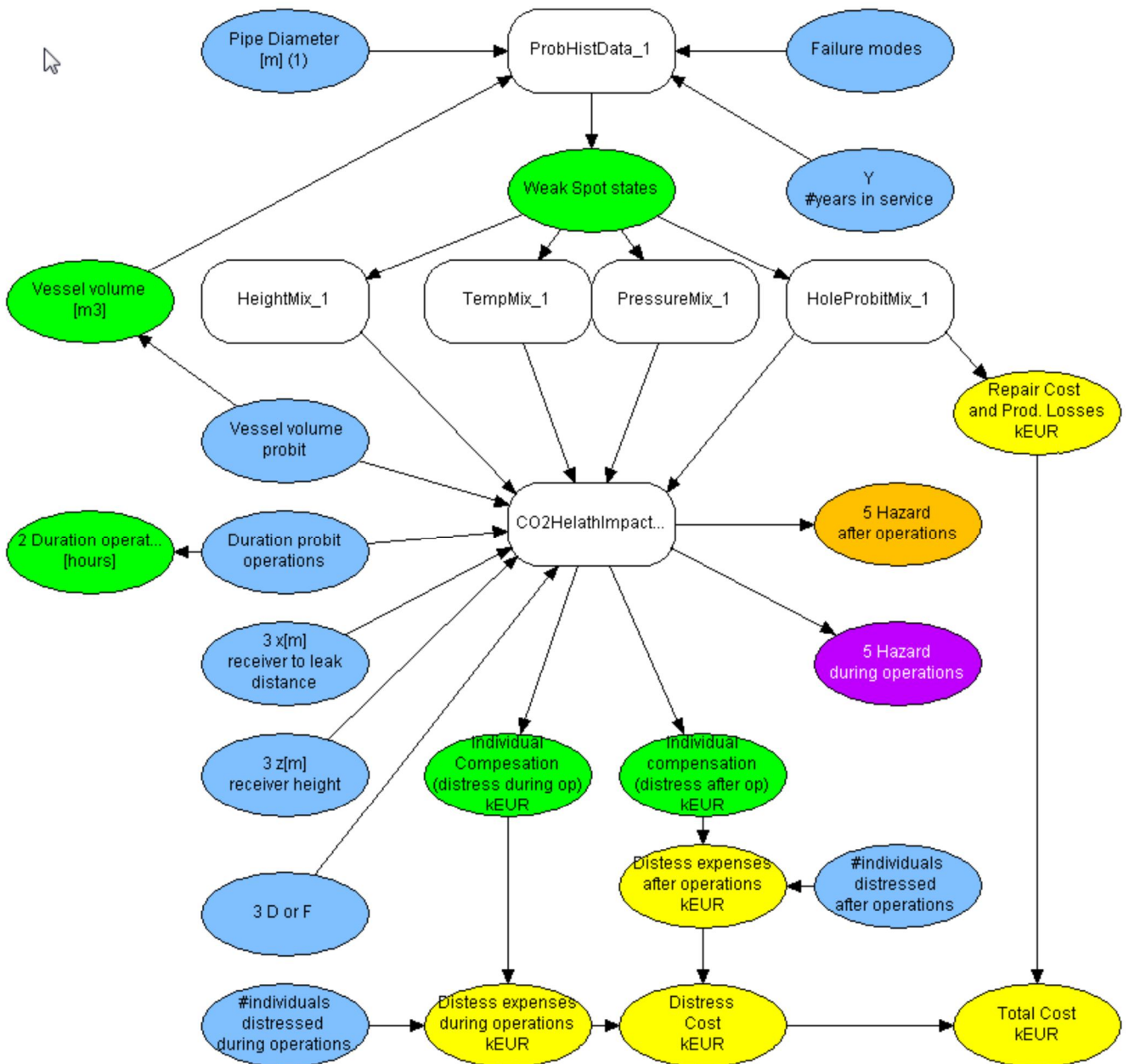
Figure 4-4 Screen capture of the main, top-level BN model showing input nodes (blue), main output nodes (yellow) and intermediate results (green, orange, purple) and imbedded sub-models (white), ref. /8/.
