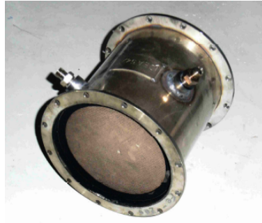
Figure 5.2: Zeolite-based SCR catalyst (Fe-ZSM5) from Johnson Matthey
