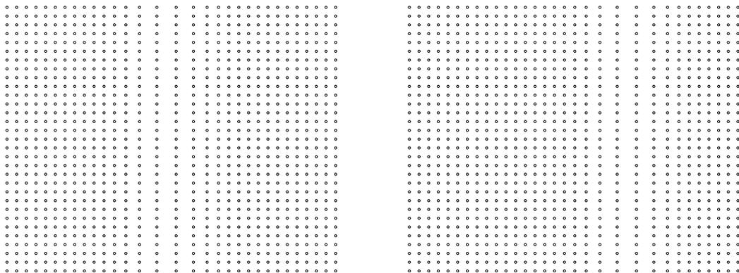
Figure 1: Particle positions for the solitary wave in the lattice with linear springs. The parameter values used here are  $K_1 = 5$ ,  $K_2 = a_1 = a_2/\sqrt{2} = 1$ ,  $(c - c_s)/c_s = 1/24$ . The solitary wave is always an extension wave and the site of the most extended cell moves along the  $(1, 0)$  direction.
