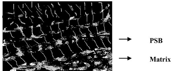
Fig. 19 Hand-sketch of Fatigue Microstructure picture originally shown in Ahmed Wilkinson and Roberts (1997)
