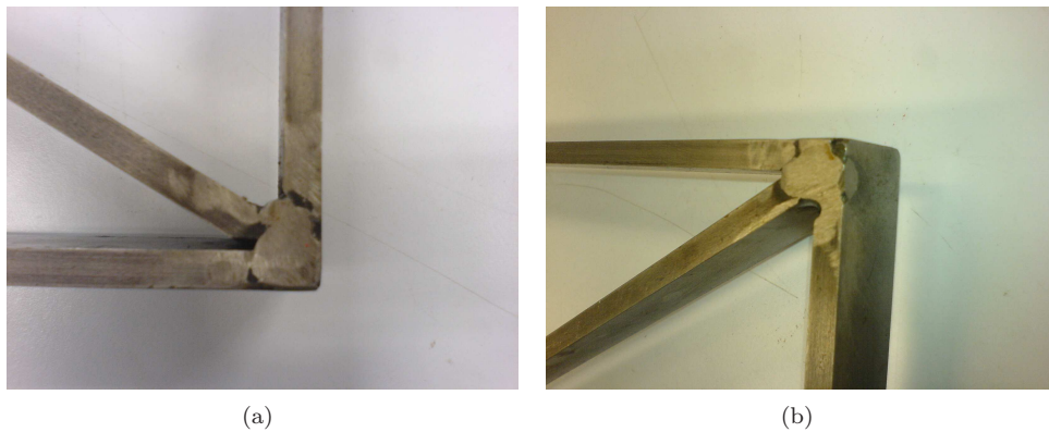
Figure 3.16: Examples of the corner joints in the welded frame.
