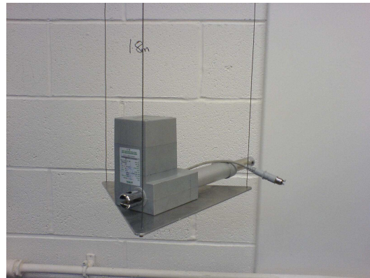
Figure C.3: The actuator sitting on the trifilar plate in the arrangement used for determining the mass moment of inertia.
