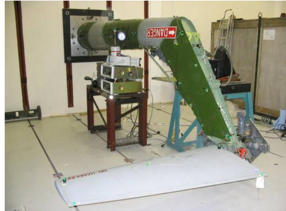
(b) Tail boom mounted on reaction wall.
