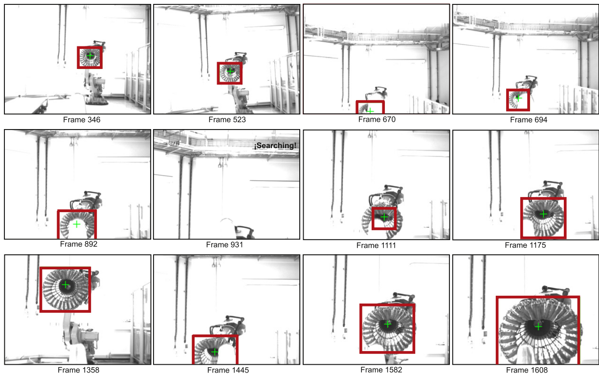
Fig. 18. Tracking results: medium turbulence. The green crosshair and red box indicate the estimated position and extent of the drogue.
