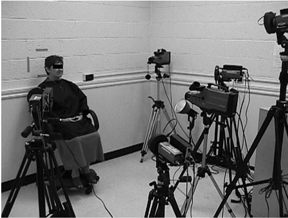
FIGURE 1. Camera configuration and set-up for recording facial movements.
