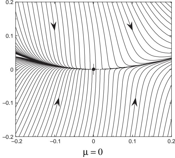
For  $|\mu| \ll 1$  trajectories decay exponentially fast towards the extended centre manifold  $y = 2\mu + x^2 + O(3)$  on which the dynamics is given by  $\dot{x} = \mu + x^2 + 2\mu x + 4\mu^2 + O(3)$ .
