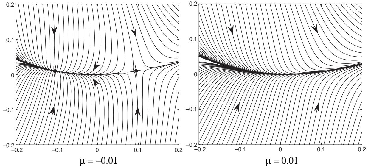
So there is a saddle-node bifurcation which creates new fixed points in  $\mu < 0$ . For  $\mu < 0$  there is a saddle at  $x = \sqrt{-\mu} + O(\mu)$  and a node at  $x = -\sqrt{-\mu} + O(\mu)$ ; for  $\mu > 0$  there are no fixed points near  $x = 0$ .
