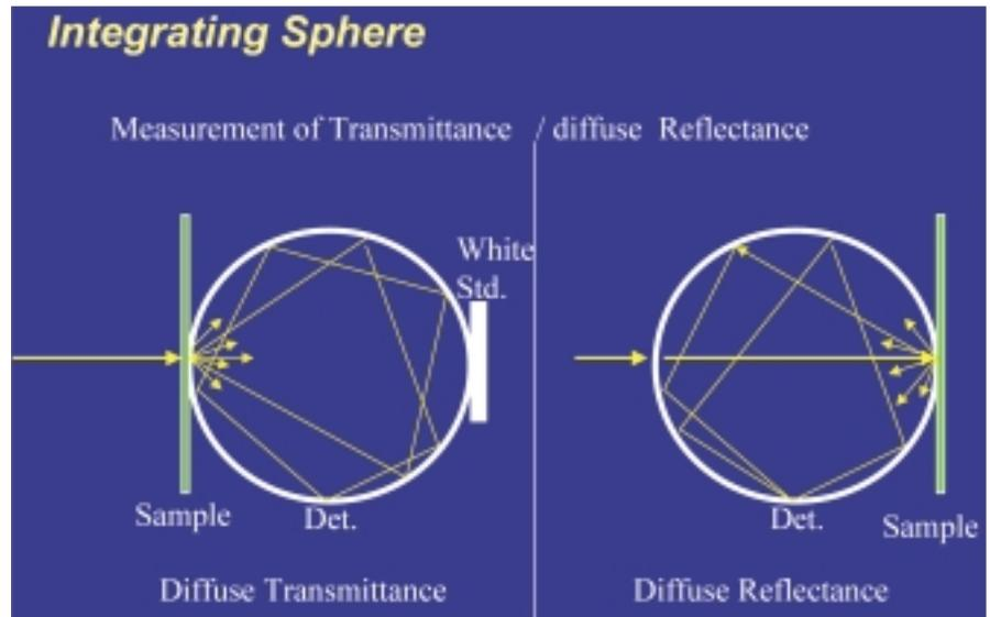
Figure 2. Measurement principles of the integrating sphere for the Lambda 35
