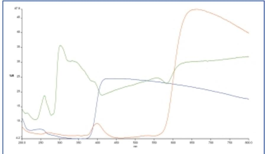
Figure 6. Reflectance spectra from 3 differently colored plastic samples measured with the Lambda 35 with integrating sphere.
