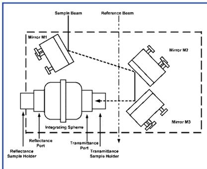
Figure 1. Optical schematics of the 50 mm integrating sphere for the Lambda 35.
