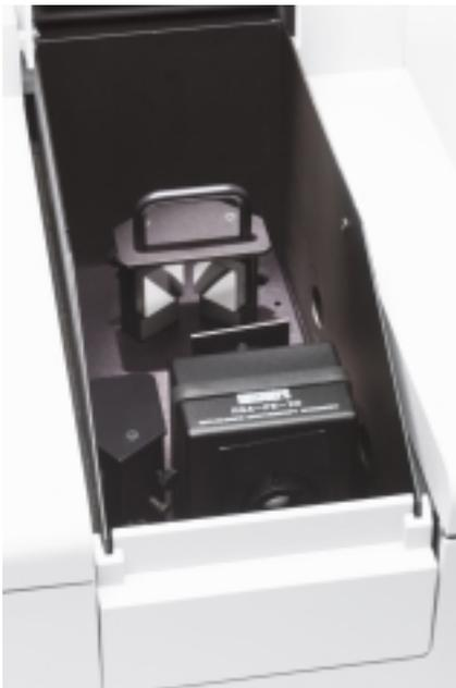
Figure 5. View into the Lambda 35 UV/Vis sample compartment with integrating sphere installed.
