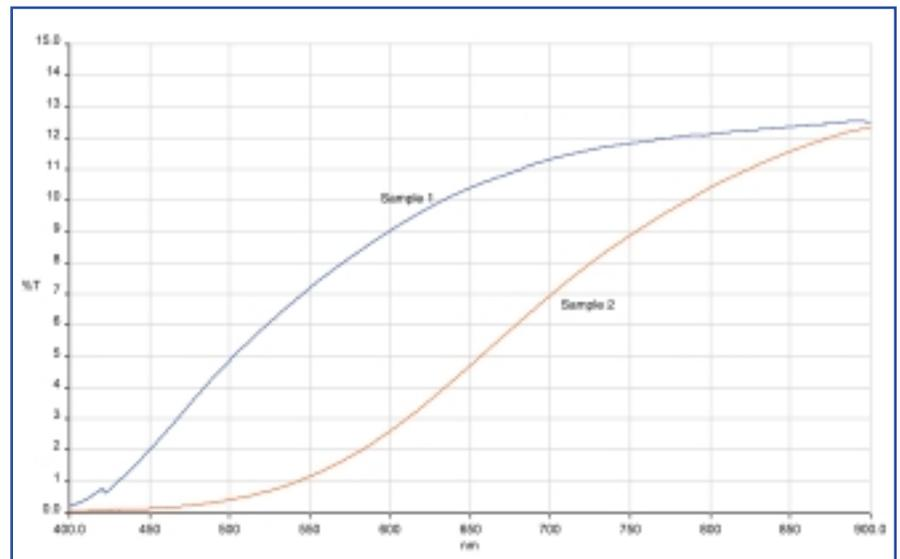
Figure 3. Average spectra of cardboard samples used as packaging material for milk. Measurement conditions; Lambda 35 with 50-mm integrating sphere. Sample in front of sphere (diffuse transmittance).
