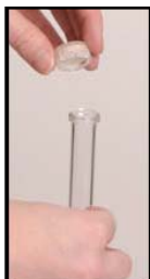
Step 1: Position cap above vessel with the notches pointing down.
