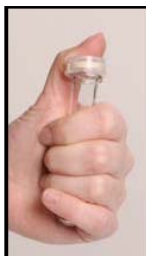
Step 2: Place cap on top of vessel at a slight angle and roll your finger over the top of the vessel.
