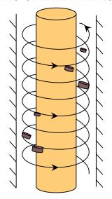
In a steady state where the drag of mud balances the gravity of cuttings:
