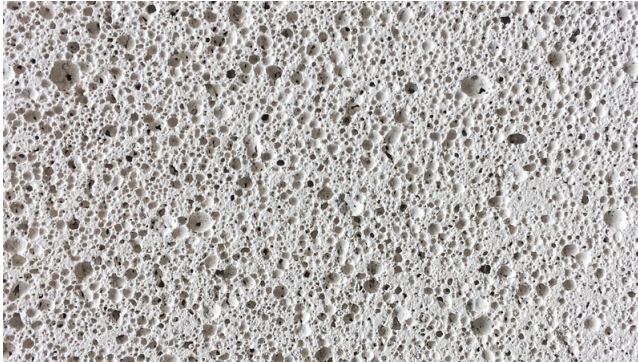
Figure: Pores in aerated concrete created by the reaction of aluminum with the binding agents lime and cement used in production. https://www.bauen.de/a/porenbeton-fuer-den-hausbau.html
