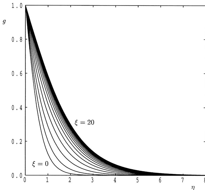
Fig. 2. Temperature profiles for various values of  $\xi$  for the case  $\gamma = 10$ . The lowest curve corresponds to  $\xi = 0$ . Successive curves correspond to  $\xi = 1, 2, \dots, 20$ .
