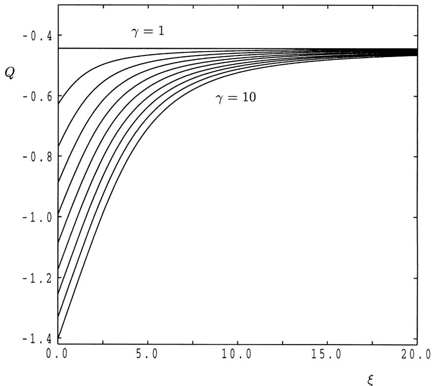
Fig. 1. Variation of the local rate of heat transfer,  $Q$ , with  $\xi$  for different values of  $\gamma$ . The straight line corresponds to  $\gamma = 1$ , the uniform permeability case. The other curves are for  $\gamma = 2, 3, \dots, 10$ .
