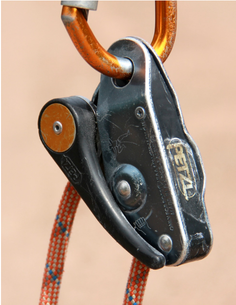
A Grigri makes a very good clutch, but adds a massive amount of friction.
