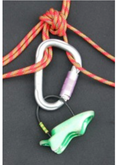
Attaching the abseil device to the spider—it is clipped through the loops attached to both climbers, i.e. across the overhand. This is the same as for a Y-hang.
