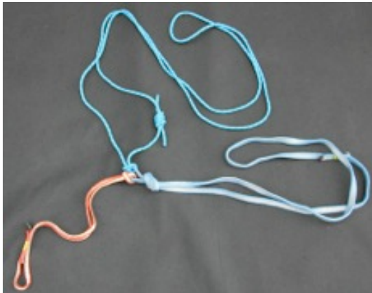
If you don't normally carry a cordelette, you can make a rescue spider from two slings and a 3m prusik loop. Or in many other ways.
