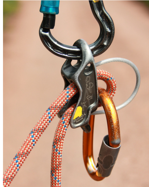
A Reverso makes a clutch that grips well with little slip back, but adds a lot of friction. With thin ropes and the casualty helping it works well (for example in an assisted hoist). It is also likely to be in place on the rope when the climber gets into trouble. So it is quick to deploy. With fatter ropes the friction is likely to be too much.
