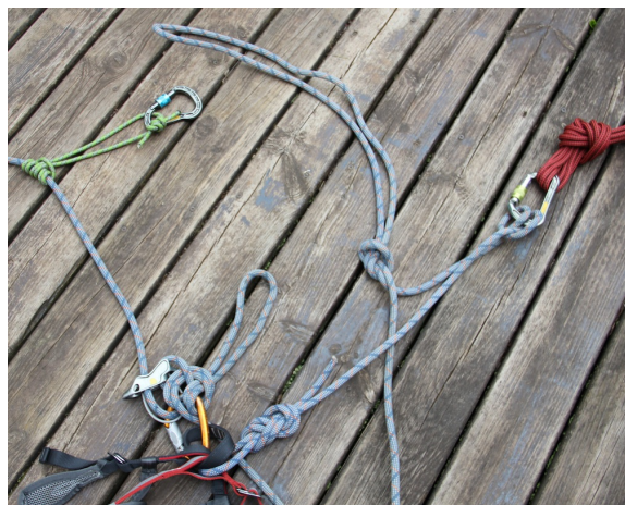
Using the spare rope on the slack side of the anchor, form a large bight of rope with an overhand.
