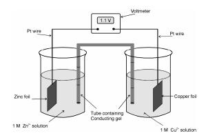
The *potential difference* between the electrodes provides the "driving force" for the electron flow.
