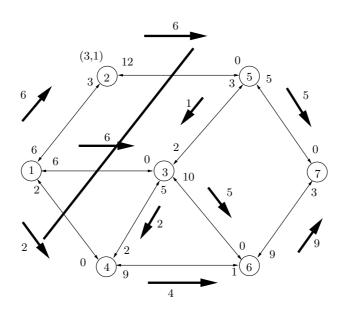
Solution 29 Constructing the diagram of the residual capacities only in the direction of the specified flows one obtains the following picture.
