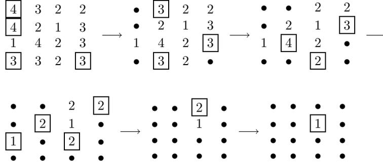
Figure 2. Illustration of the burning algorithm on a  $4 \times 4$  lattice. At each step, framed sites are burnt.
