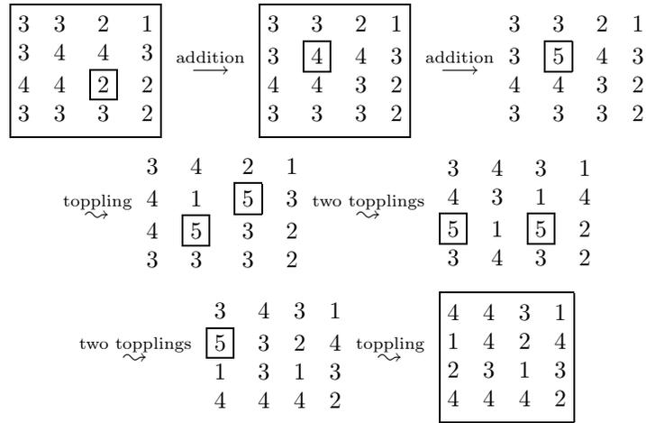
Figure 1. Illustration of the dynamics on a  $4 \times 4$  lattice. Framed configurations are stable. Framed sites represent particle addition or toppling. The second particle addition results in an avalanche of 6 topplings.
