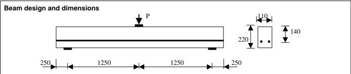
Concrete cube strength  $f_{cu} = 53.3 \text{N/mm}^2$ , tensile strength  $f_t = 5.74 \text{N/mm}^2$ . Two steel tendons of 7mm  $\phi$  each snap at  $f_{pu} = 1750 \text{N/mm}^2$ . Effective prestress 57% of  $f_{pu}$ . Young's Modulus  $E_s = 200,000 \text{N/mm}^2$  for steel and  $E_c = 30,000 \text{N/mm}^2$  for concrete
