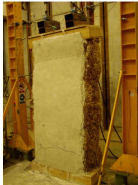
Figure 8 Lime rendered wall failure
