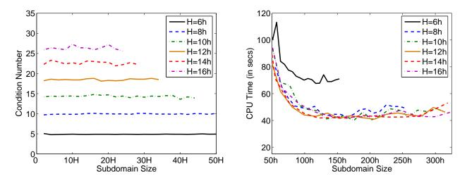
Figure 4: Condition numbers and CPU times for Laplacian ( $n=1024^2,\,\delta^{sub}=3h,\,\mu=1$ ).
