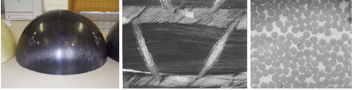
FIGURE 1. A hierarchy of textile structures from left to right: the composite part (1 m), the fabric (0.01 m), the fibres (0.0001 m). [Pictures: S. Lomov].
