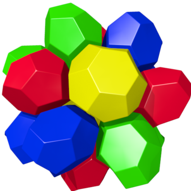
Figure 3: The unit cell of the new partition P42a contains 14 polyhedra of 4 different kinds. Four 1-10-2 (red), two 0-12-2 (yellow), four 1-10-3 (green) and four 2-8-4 (blue).
