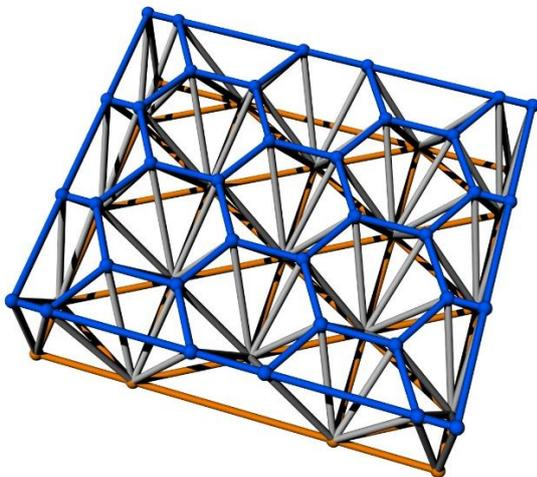
Fig. 6 Original layer (blue), connected (in grey) to its dual (orange)
