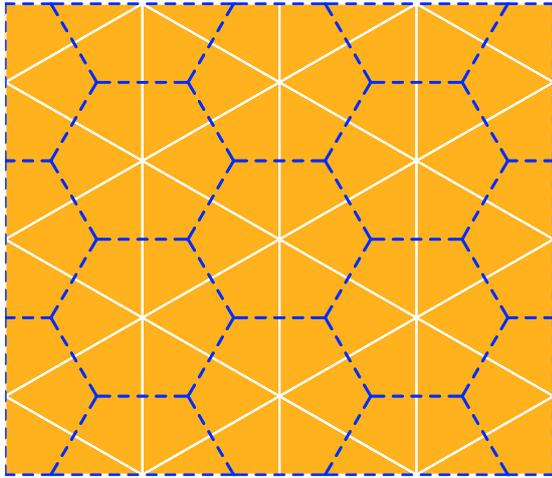
Fig. 1 Original hexagonal mesh (blue dashes) with its dual (orange)
