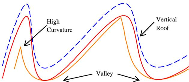
Fig. 5 An original structural layer (blue dashes) with its vertical offset (red) and normal offset (orange)
