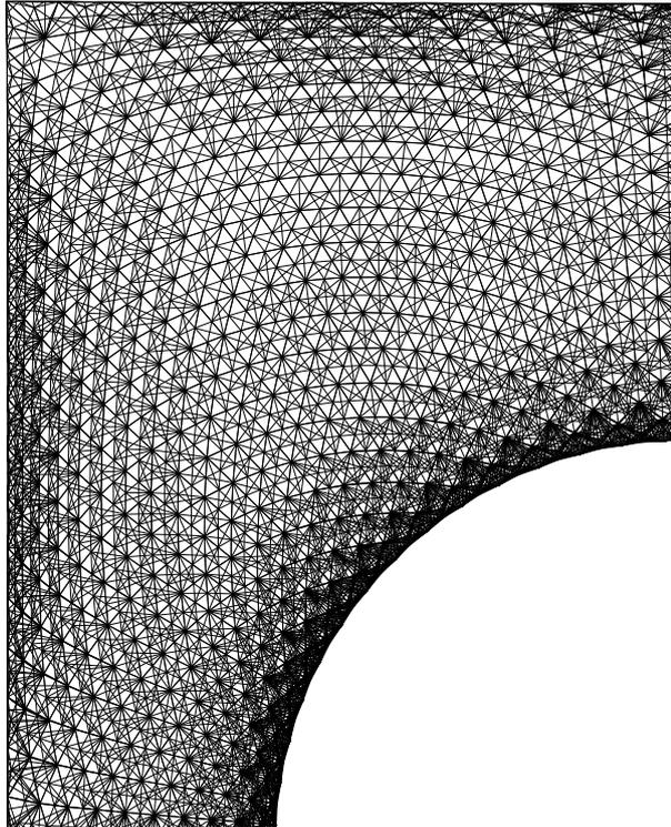
Fig. 9 Initial Ground Structure used for Optimization
