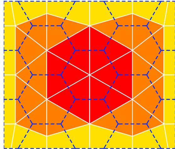
Fig. 7 Initial hexagonal mesh (blue dashes) and its triangular dual showing internal faces unaffected by the boundary (red), slightly distorted (orange) and special-case boundary faces (yellow).
