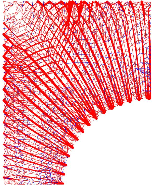
Fig. 10 Optimized layout showing compression (red) and tension (blue) where line-thickness represents the level of stress in a member
