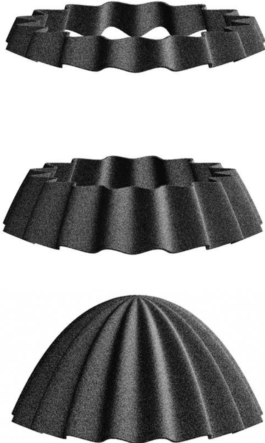
Figure 3: Peridynamic model of a concrete shell during printing
